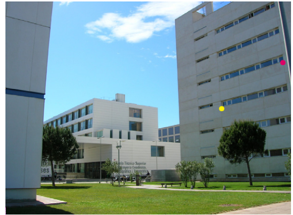
Fig. 4. Circular coloured elements acting as control points for the tracking in real time.
